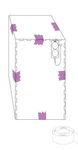
Secure the entire box and the external parts with tape while the glue dries.
