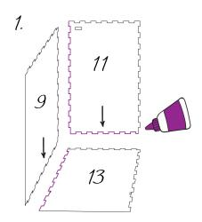
Glue the left wall, floor and box ceiling together (parts 9, 11 13)
