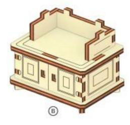
4. Insert the two parts numbered 5 into the bottom of part 3 as shown above. Attach that to the top of the assembly.
