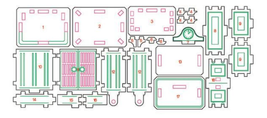
2. Insert the four parts numbered 4 into the bottom of part 2 as shown above. Attach one of the parts numbered 9 to part 8 and part 18. Attach the other part numbered 9 to the other side of parts 18 and 8. This will be called assembly A.
