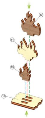
Fit piece 13 (foreground), piece 11 (middle), and piece 12 (background) into slots of piece 18 as shown to construct "A" group
