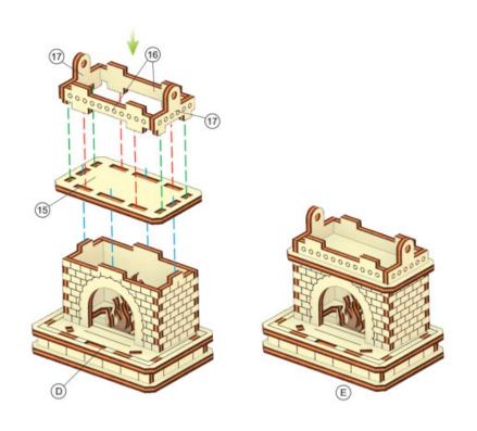
Fit piece 15 to tabs of group "D" as shown. Fit pieces 16 and 17 to slot
