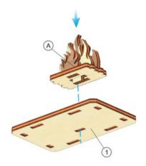
If assembling lighting - piece 1 will have a strip cut out. trail the wires from the led diode light through this strip and continue regular assembly. Use glue as needed to secure the diode and wires.
