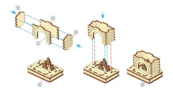
Fit brick wall pieces 3, 8 and 9 to slot holes of group "C" to make group "D"
