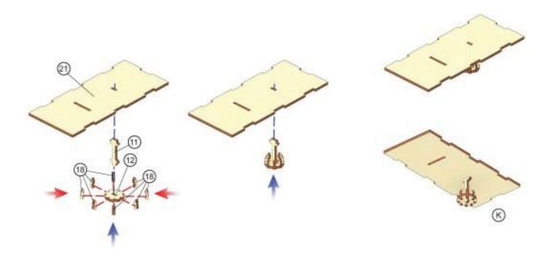
Attach the ceiling to the top of the assembly.
