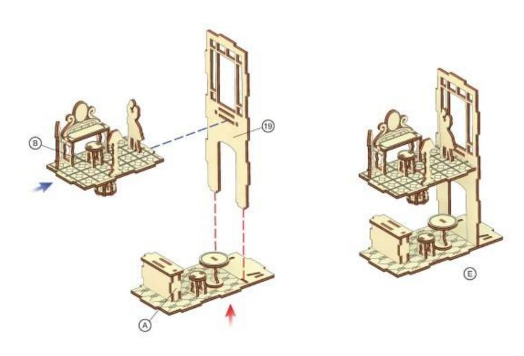
Attach the back wall, the base, front steps and front door
